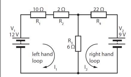
$V_1$  is supplied from a variable power supply that is supplied with a current of 1.1 amps.
