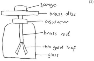
Use an electroscope. Put the sponge on the brass disc. If the sponge is thouged, the two pieces of thin gold leafs would move away from each other.
