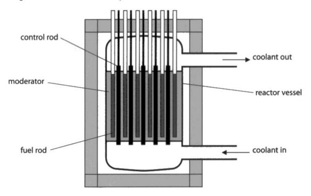
(a) Describe how a chain reaction occurs in a nuclear fission reactor.
