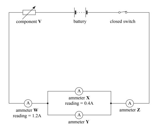
blank (i) Identify component V. **(1)** (ii) State the reading in amps on  $\text{ammeter } \boldsymbol{Y}$ reading =  $\dots$ A reading = .....A ammeter  $\mathbf{Z}$ **(2)** (d) The following circuit diagram shows how a toymaker connects the lights in a toy house. (i) Complete the sentence. The lights in the toy house are connected in ..... **(1)** (ii) Suggest one advantage of connecting the lights in this way. **(1) Q8** (Total 8 marks)
