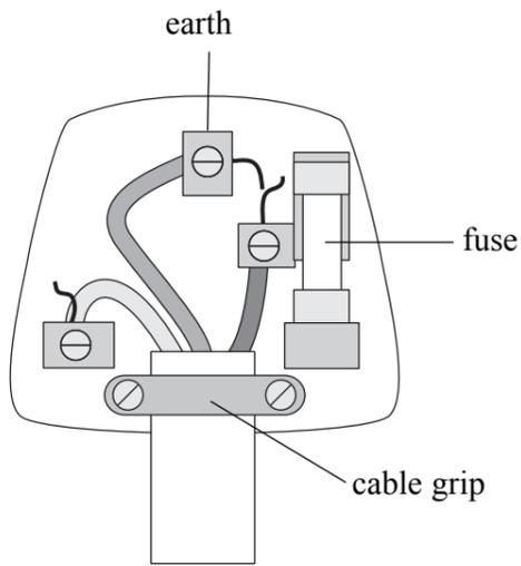
The cable is secured by the grip so that it cannot be pulled out of the plug.
