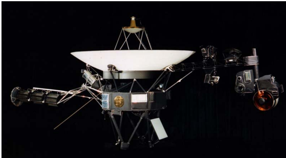
Figure 7: The Voyager Probes. Launched in 1977, these two spacecraft used the gravity of the Earth, Sun and Jupiter to become the first probes to take photographs of the outer solar system. Their paths were not 'closed' orbits and so they have both now left the Solar System, never to return... (Image: ©NASA)
