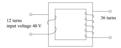
(i) Calculate the value of the output voltage.
