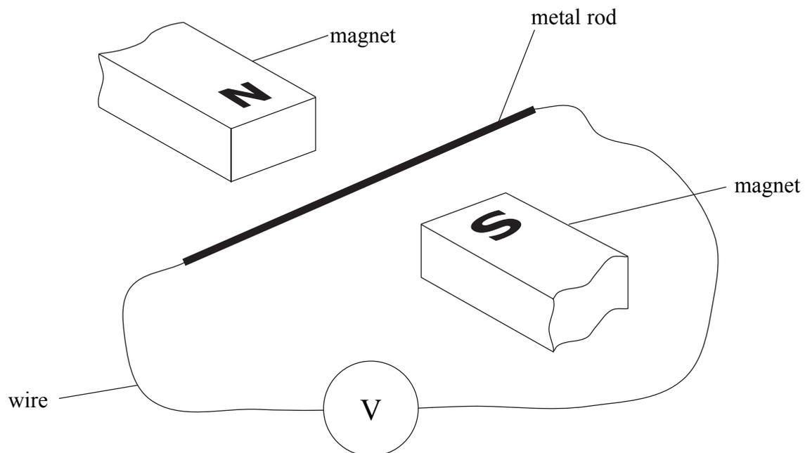
She moves the metal rod upwards and the voltmeter briefly shows a small reading.
