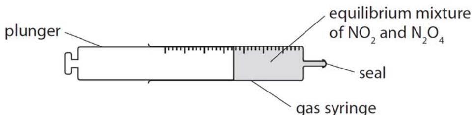
The plunger is pulled out to reduce the pressure of the gaseous equilibrium mixture. The colour of the mixture first of all changes to light brown as it now occupies a larger volume. However, it then goes darker brown in colour as a new equilibrium is established.
