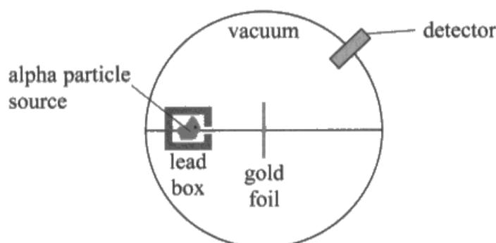
(a) Explain why the alpha source was placed in a lead box with a single small hole.
