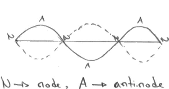
Burn marks appear where intensity of microwaves is maximum, due to superposition, i.e. at an anti-node (A). Distance between two successive burn marks is distance between two successive anti-nodes, ~~which is~~ which is half of wavelength. Therefore, wavelength is twice the distance  $\Rightarrow \text{Distance} (d) = \frac{\lambda}{2} \Rightarrow \lambda = d \times 2$ .
