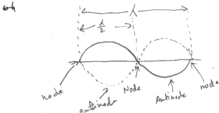
In standing waves, there are points called nodes, where energy is minimum, and antinodes, where energy is maximum. Burns occurs when there ~~is one~~ <sup>is an</sup> antinode (maximum heat energy). And, the distance between two adjacent antinodes is half the wavelength. That is why wavelength of microwave is twice the distance between the <sup>burn marks</sup> a
