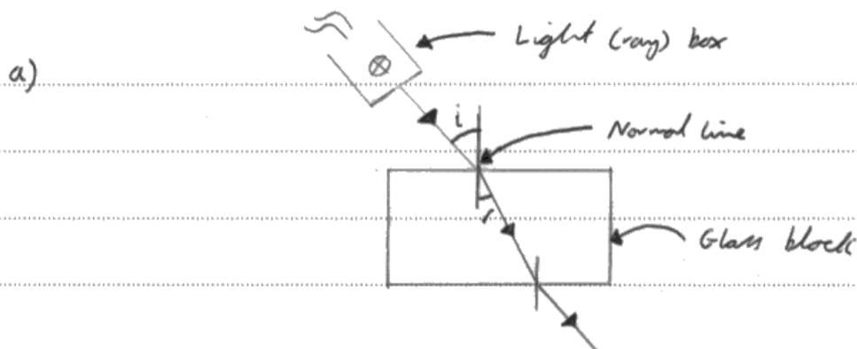
A ruler, pencil, protractor and power supply will also be needed. A sheet of paper ~~may~~ may be placed under the glass block to trace the rays of light.
