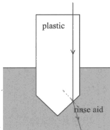
Complete the diagrams to show the paths of light when the rinse aid level is low and when it is high.
