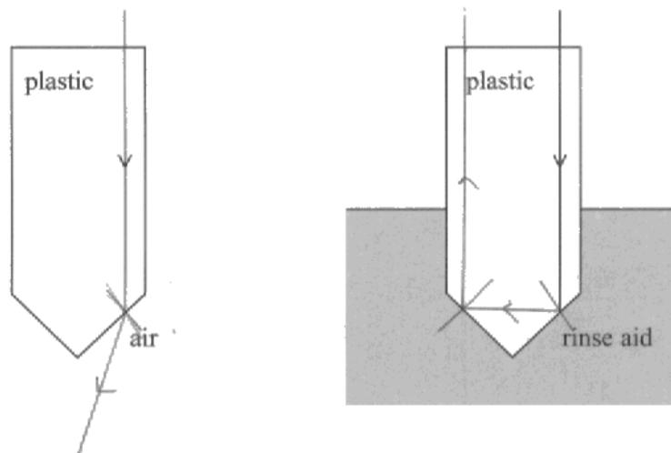
Complete the diagrams to show the paths of light when the rinse aid level is low and when it is high.
