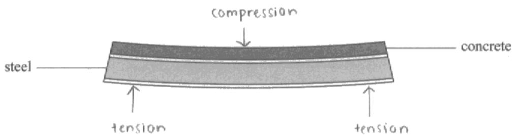
(a) (i) Label the diagram to show where the beam is under tension and under compression.
