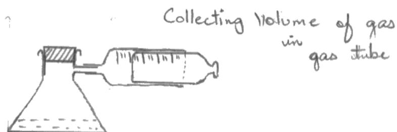
Because one of the products is gas. We can use collect volume of gas to know ~~the~~ rate of reaction. Known amounts of reactants added and volume collected is noted. Repeat, a couple of times and then calculate rate of reaction from known values.
