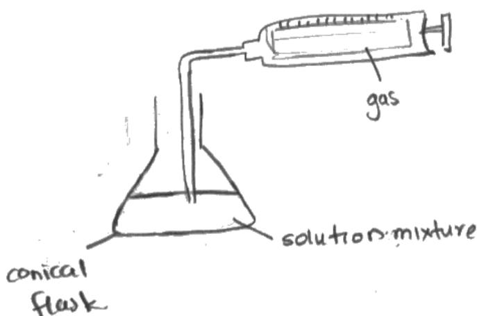
Use a syringe to find the volume of the gas and the rate of reaction. Take a sample of solution of compound A in a flask and add compound solution B into it. Then the gas will be collected in the syringe.
