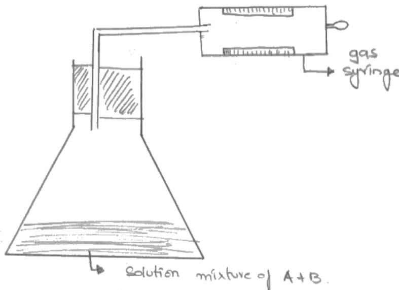
Compound A and B is placed in a flask. The flask should be connected to a gas syringe (as shown). The volume of gas released should be recorded at regular time intervals. After attaining sufficient values of the volume of gas collected at regular time intervals a graph of volume of gas C against time should be plotted. ~~The gradient of the~~ The shape of the graph obtained from the result would tells us about the rate of reaction.
