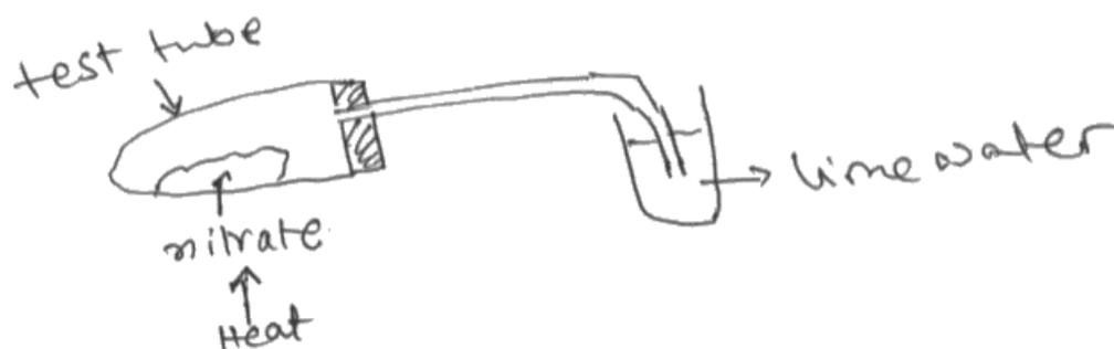
Time for lime water to turn milky is measured for both nitrates, <sup>to compare.</sup> Here, volume of lime water and mass of nitrate with constant flame distance from tube should be maintained for a fair test.
