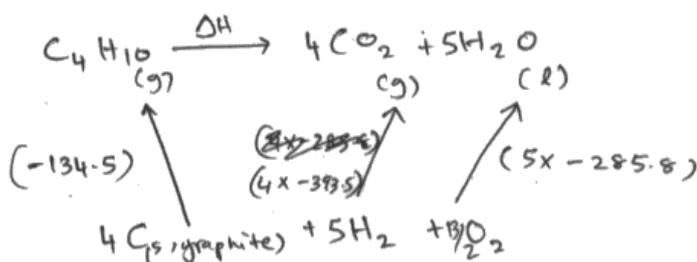
$$\begin{aligned} \Delta H + (-134.5) &= (4 \times (-393.5)) + (5 \times -285.8) \\ &= (-1574) + (-1429) \\ &= (-3003) + 134.5 \\ &= -2868 \text{ kJ mol}^{-1} \end{aligned}$$
