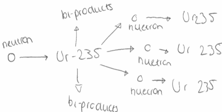
A neutron is fired at Uranium 235 which then causes two bi products to be made (these are usually krypton and barium but they can be different) Also two or three neutrons are made which means that they could collide with more uranium for more ~~the~~ reactions.
