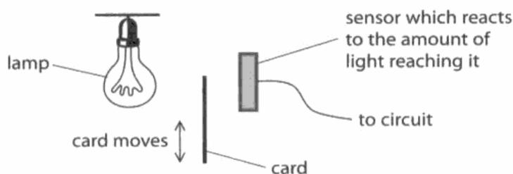
The piece of card can be moved up and down between the lamp and the detector. Each part of the teacher's arrangement corresponds to a part of the machine.
