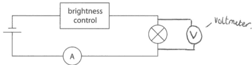
(i) Add a voltmeter to the circuit which will measure the potential difference (voltage) across the lamp.
