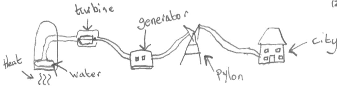
the heat from a nuclear reactor heats water and forms steam. The steam then rises and turns a turbine as the turbine spins electrical energy will be produced in a generator and get transferred to the pylons and then to a city
