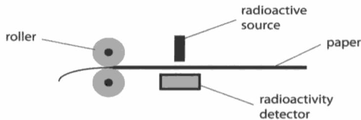
The radioactive source used must be chosen carefully to be effective and used in a way that is not a hazard to workers.
