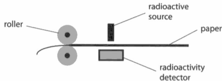
The radioactive source used must be chosen carefully to be effective and used in a way that is not a hazard to workers.
