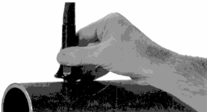
The ultrasound wave travels through the metal and is reflected at the inner surface of the metal.
