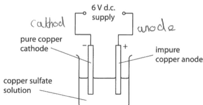
Describe and explain what is seen when this apparatus is used to purify a piece of impure copper.
