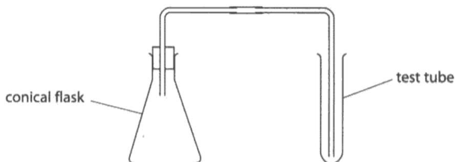
You can use this equipment by putting/mixing the sodium carbonate and dilute acid together in the test tube. They will react and produce a gas which will travel along the tubing and into the conical flask where it can be tested for to reveal if it is  $\text{CO}_2$  or not.
