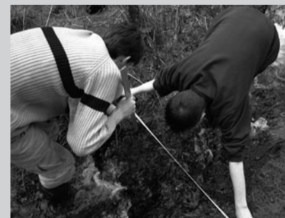
Measuring wetted perimeter (above) and channel width (below)
