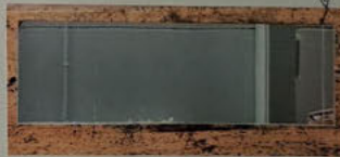
also cut with laser cutter mirror was not long enough so small one on the side had to be cut and stuck on the side of the panel
