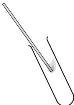
The test to see if a gas is oxygen is: a glowing splint of wood will re-light.
