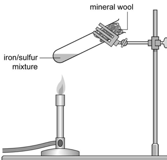
2. Clamp the tube at the top at an angle. Heat the tube strongly near the middle as shown.
