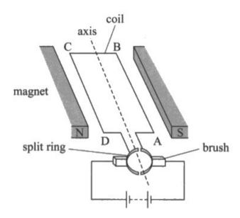
\*(a) Describe how this arrangement can lead to the coil rotating.
