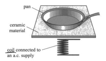
(a) A steel pan containing water is placed on the induction hob.
