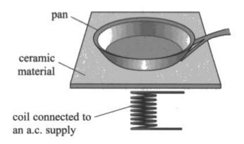
(a) A steel pan containing water is placed on the induction hob.
