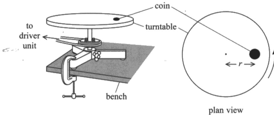
(a) The student measured the distance  $r$  between the centre of the turntable and the centre of the coin, with a metre rule as shown.
