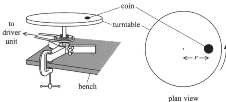
(a) The student measured the distance  $r$  between the centre of the turntable and the centre of the coin, with a metre rule as shown.
