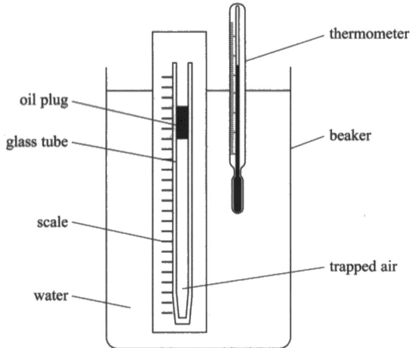
A glass tube was sealed at one end. A plug of oil trapped a length  $l$  of air in the tube. The water in the beaker was heated to a temperature  $\theta$ . The corresponding value of  $l$  was measured. This was repeated for a range of temperatures.
