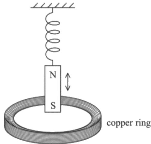
The magnet is displaced vertically and released so that it oscillates.
