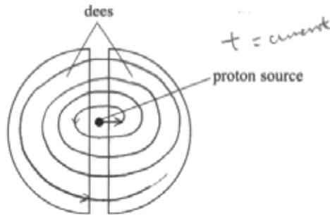
(i) Complete the diagram to show the path of the protons.
