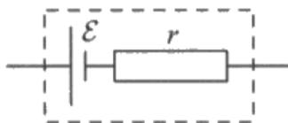
A student used the relationship  $V = \mathcal{E} - Ir$  and a graphical method to determine  $\mathcal{E}$  and  $r$ . She connected a cell in a circuit and took a series of measurements of the current  $I$  in the cell and the potential difference  $V$  across the terminals of the cell.
