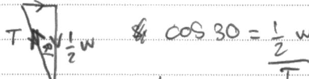
The diagram shows a vertical line representing a leg. A horizontal arrow labeled 'T' points to the right from the top of the leg. A vertical arrow labeled '1/2 W' points downwards from the top of the leg. A diagonal line representing the leg is drawn from the top of the vertical line downwards and to the right, forming a 30-degree angle with the vertical. The text  $\cos 30 = \frac{1/2 W}{T}$  is written next to the diagram.
