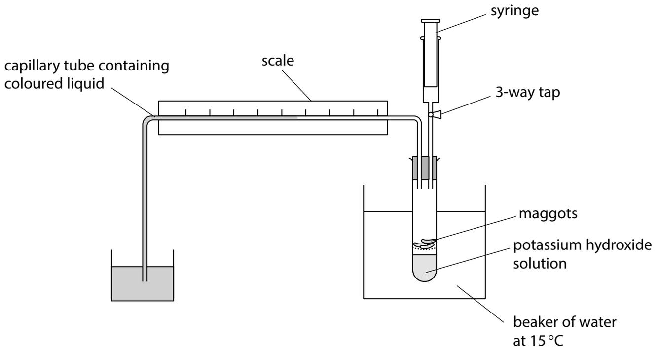
Maggots were placed in the boiling tube and the 3-way tap was closed.
