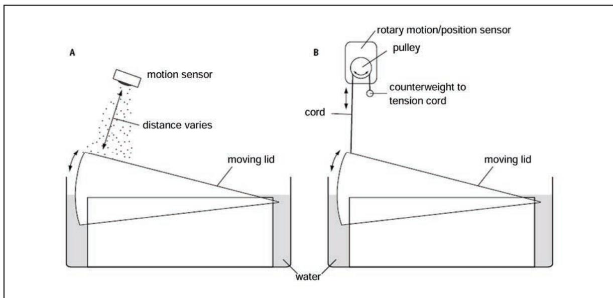
Figure 1 Motion sensors fitted to a spirometer.
