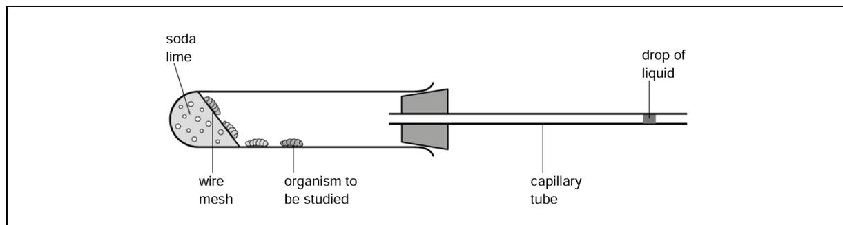
**Figure 1** A very simple respirometer.
