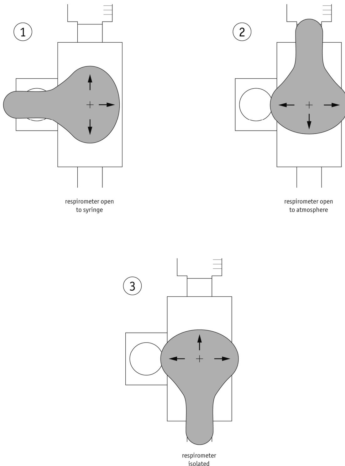
Figure 1 Tap positions for a three-way tap (viewed from the side).
