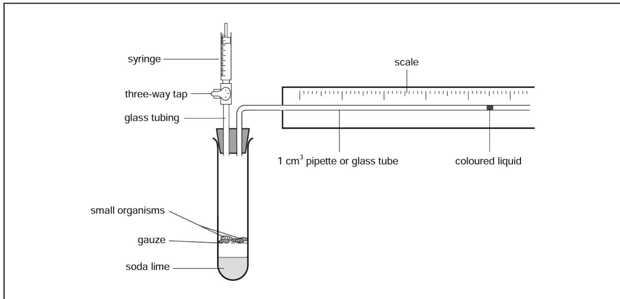
**Figure 2** A simple respirometer using a boiling tube.
