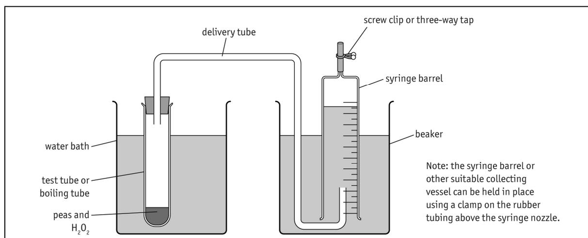
**Figure 1** An example of apparatus set up to measure the volume of gas evolved.
