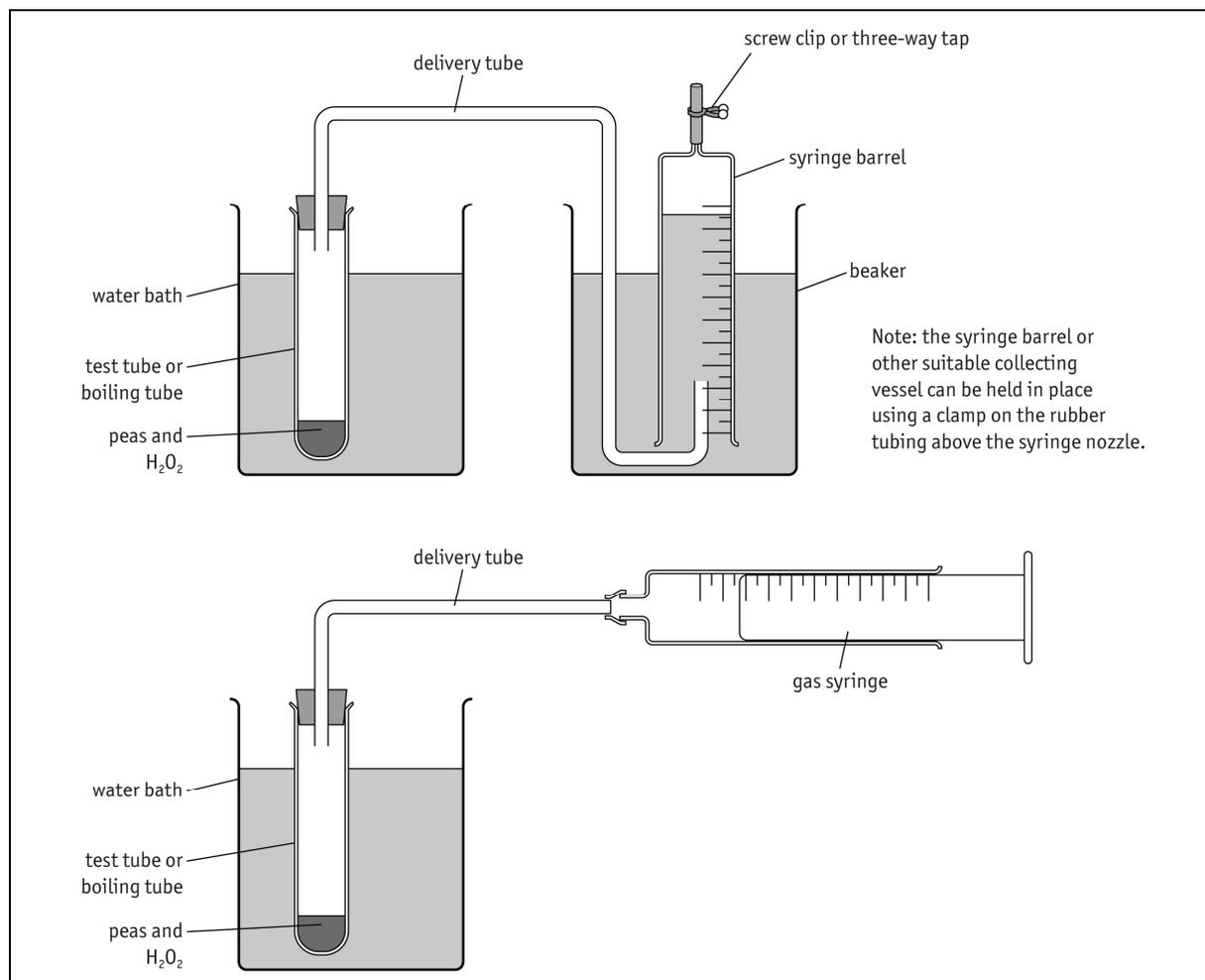
**Figure 1** Examples of apparatus used to measure the volume of gas evolved.
