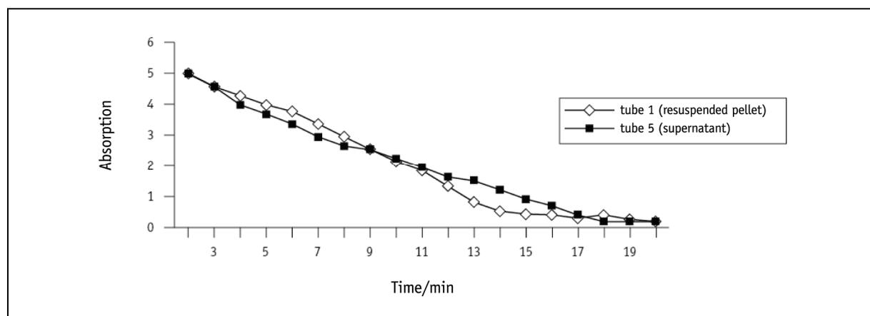
**Figure 1** Results using bench centrifuge. DCPIP chloroplast extract spun for 10 minutes at  $95\times g$ .
