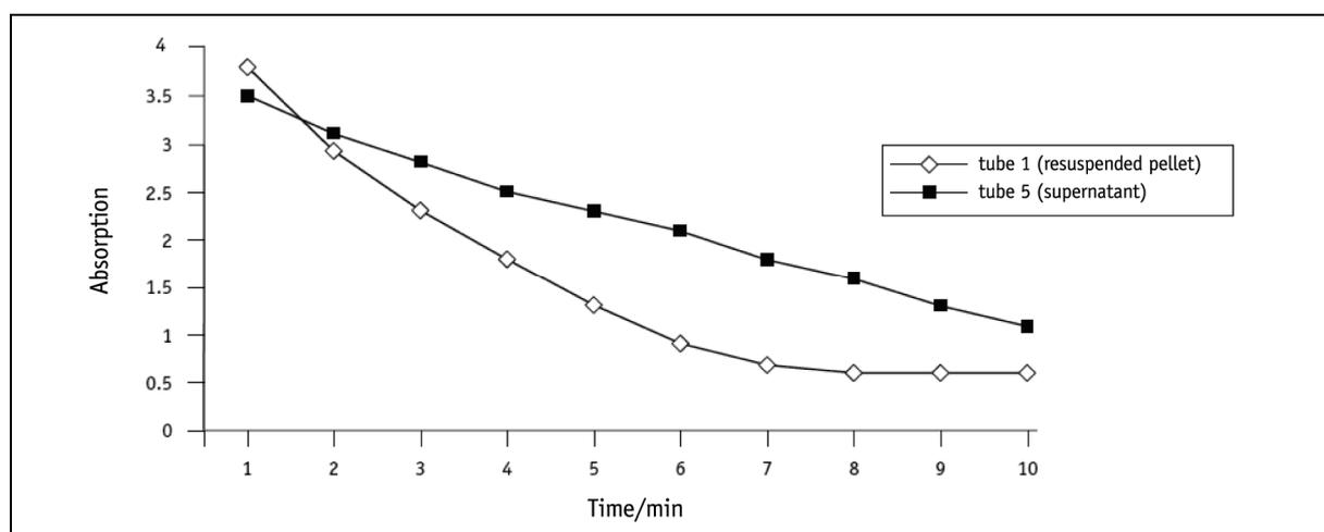
**Figure 2** Results using micro-centrifuge. DCPIP chloroplast extract spun for 5 minutes at 2000× g.
