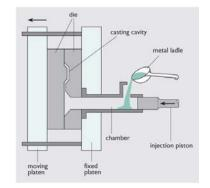
Pressure die casting is a development of gravity die casting in which molten metal is injected into a steel mould under pressure; it is the metal equivalent of injection moulding.
