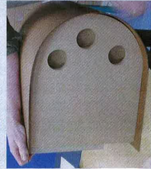
8 sheets of hardboard were bent around the mould. Each sheet was glued to the one below it.
