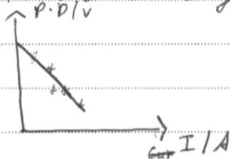
Using the graph and equation of terminal voltage the y intercept will be the e.m.f of the cell and the gradient of the graph will give the internal resistance  $r$ .
