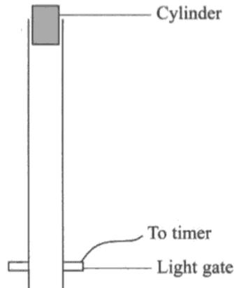
(b) The student needs to determine the velocity  $v$  of the cylinder as it passes through the light gate.
