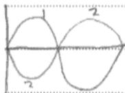
The waves 1 and 2 are in antiphase, the sum of these waves at any point will (provided they are of equal amplitude) equal zero, completely cancelling out each other. This is destructive interference.
