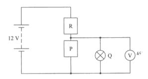
The supply has a negligible internal resistance. The reading on the voltmeter is 4.0 V.
