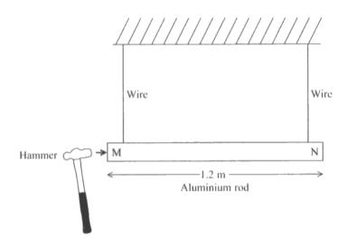
A wave pulse is made to travel along the rod and reflect from end N. The wave pulse is produced by hitting end M gently with a hammer so that the hammer remains in contact with end M until the reflected pulse returns.
