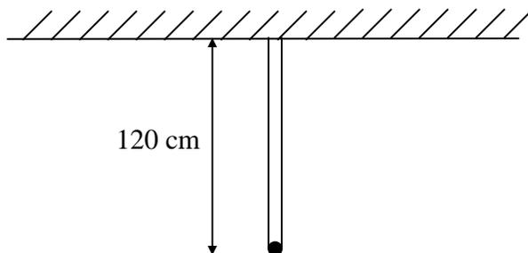
A particle of mass 5 kg is attached to one end of two light elastic strings. The other ends of the strings are attached to a hook on a beam. The particle hangs in equilibrium at a distance 120 cm below the hook with both strings vertical, as shown in Fig. 1. One string has natural length 100 cm and modulus of elasticity 175 N. The other string has natural length 90 cm and modulus of elasticity  $\lambda$  newtons.
