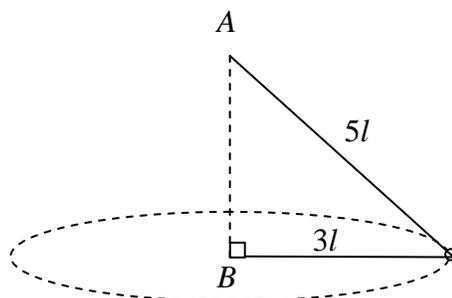
A light inextensible string of length  $8l$  has its ends fixed to two points  $A$  and  $B$ , where  $A$  is vertically above  $B$ . A small smooth ring of mass  $m$  is threaded on the string. The ring is moving with constant speed in a horizontal circle with centre  $B$  and radius  $3l$ , as shown in Fig. 2. Find
