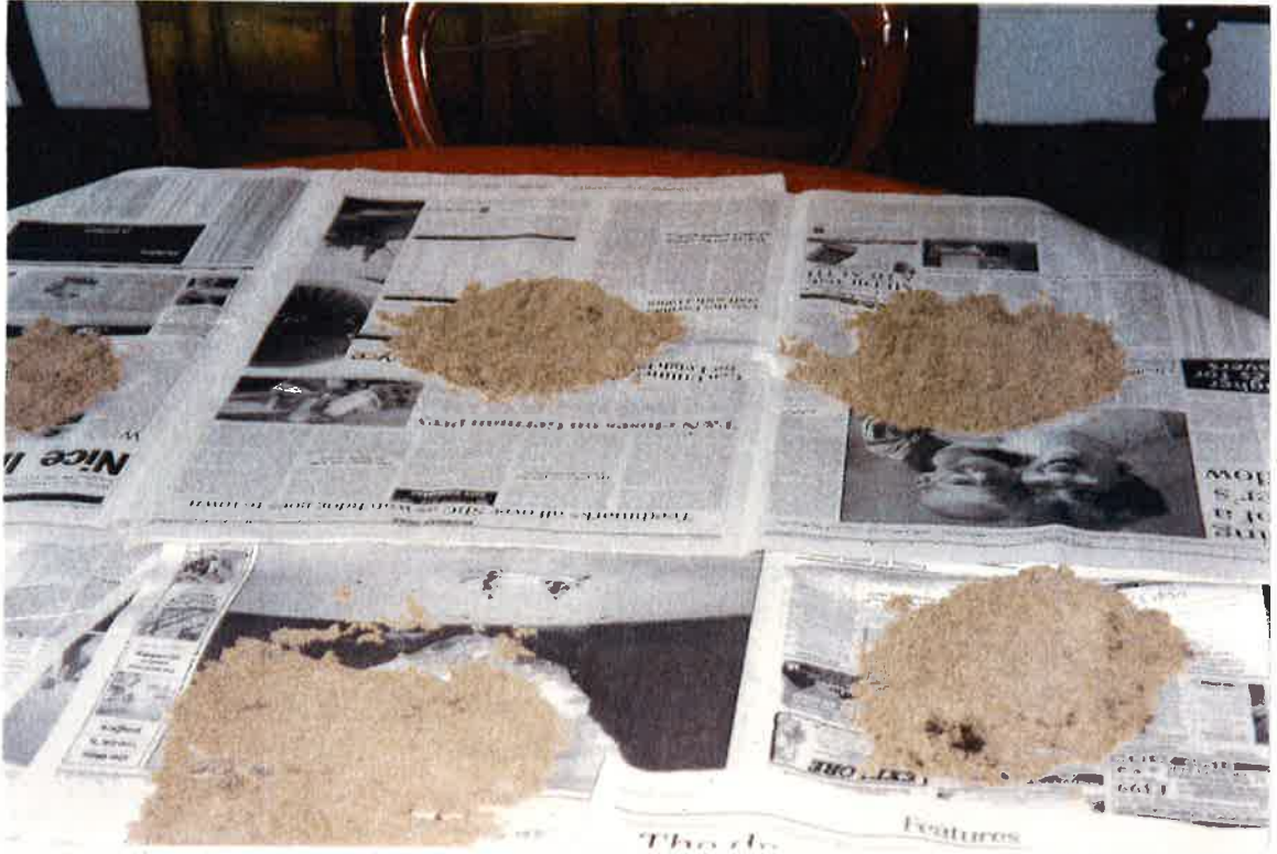
Beach sediment being dried before weighing
