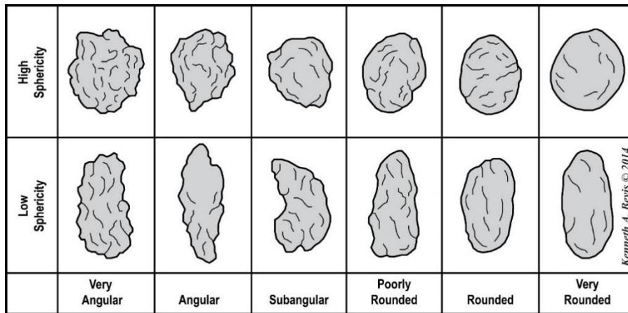
Figure 41: A table showing grain shape; sedimentary particles become more rounded and spherical as they are transported
