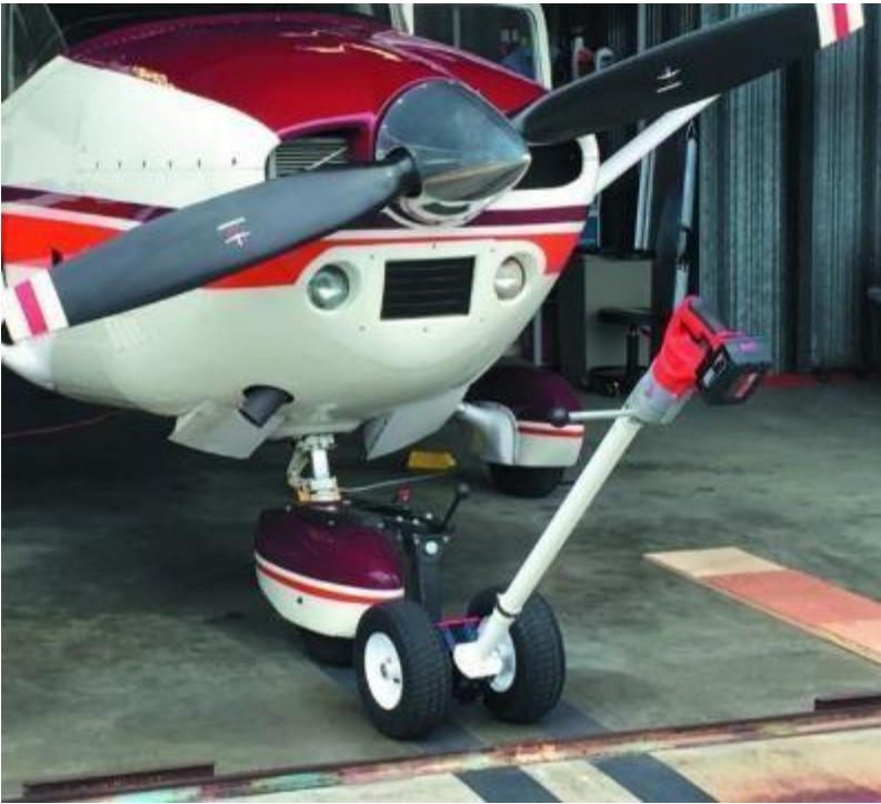
Above: Example aircraft tug. Note the steep angle of the towing arm to allow the user to pull with ease
