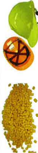
Fig. 1. ABS plastic in pellet form.
