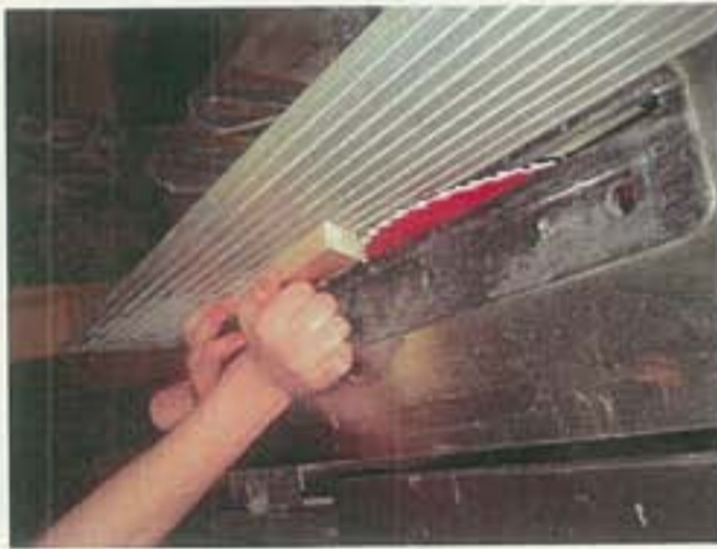
I then asked the teacher to cut my groove using the circular saw as boys are not allowed to use this machine as it is to dangerous.
