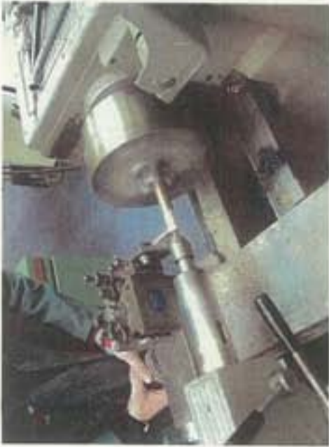
The last process is always parting off. We part off to divide the work from the rest of the material.
