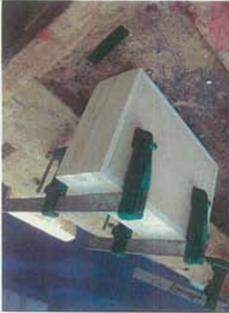
Once the box had dried I fitted the rebate joint with 3mm MDF cut to size. This was tricky and involved using a chisel to level off some of the edges.
