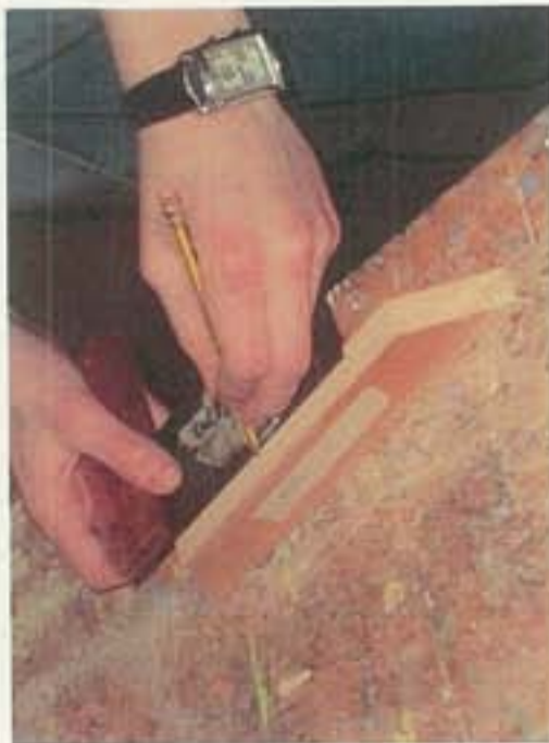
I then marked out the groove using a marking gauge and a tri square. This was easy as after I had marked one the other followed the same line on the circular saw so it was not necessary to mark them all.
