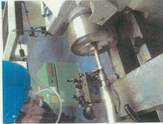
The diamond knurling was done with a knurling tool at a lower speed than before.
