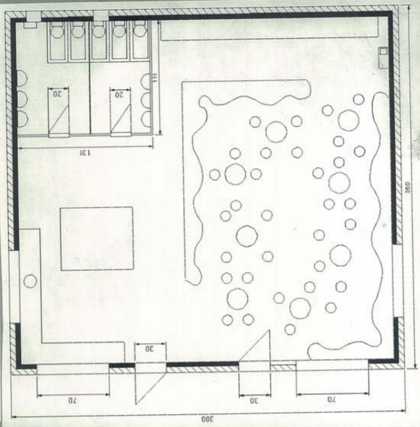
This is a floor plan of the bottom floor with measurements of the main structure. It also shows the structure of the outer walls with the breeze blocks and main bricks. I chose not to include the outdoor area that comes off of the side, but this fits exactly into the space given. This will help me when I start making the
