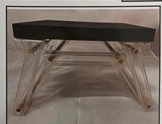
To ensure the table was lightweight and moveable, the legs and support under the table were created using square acrylic pipe instead of wood. To ensure that one element of the lack table was still part of the design, the original table top was kept.
