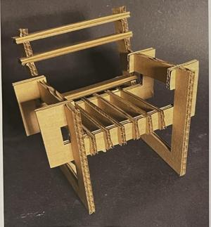
In this design, I transitioning from card to cardboard and noticed that there needs to be more slots for the backrest as they need to be closer together to compose a more complete chair.
