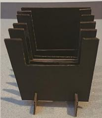
For this development I reduced the angle between the seat and the backrest to enhance the comfort of the seating position. In addition to this I added another shorter length slat at the back of the seat to ensure a lower incline on the seat.
