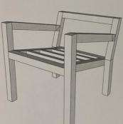
The structural necessities in this design are the front legs and apron and the rear legs and lower rail of the chair. This allows the chair to be constructed easily.
