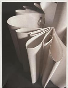
Experimenting With Sharp Folded Segments To Improve The Collapsibility Of The Paper Structure
